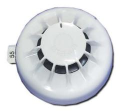
The 800H is a flexible cost-effective addressable heat detector with all the features of MX VIRTUAL detectors. The 800H returns the temperature to the MX detection panel which allows various detection modes to be implemented. The 800H uses a high quality thermistor with very low thermal mass. This allows the detectors to provide fast accurate temperature detection as well as heat detection.
