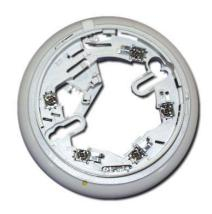
With all the features of the 5B Universal Base the 5BI Isolator Base allows any or all 800 Series MX Detectors to be upgraded to incorporate bi-directional short circuit isolation. Implemented on every detector, the 5BI can ensure that no detector is lost on a system in the event of an open or short circuit.
